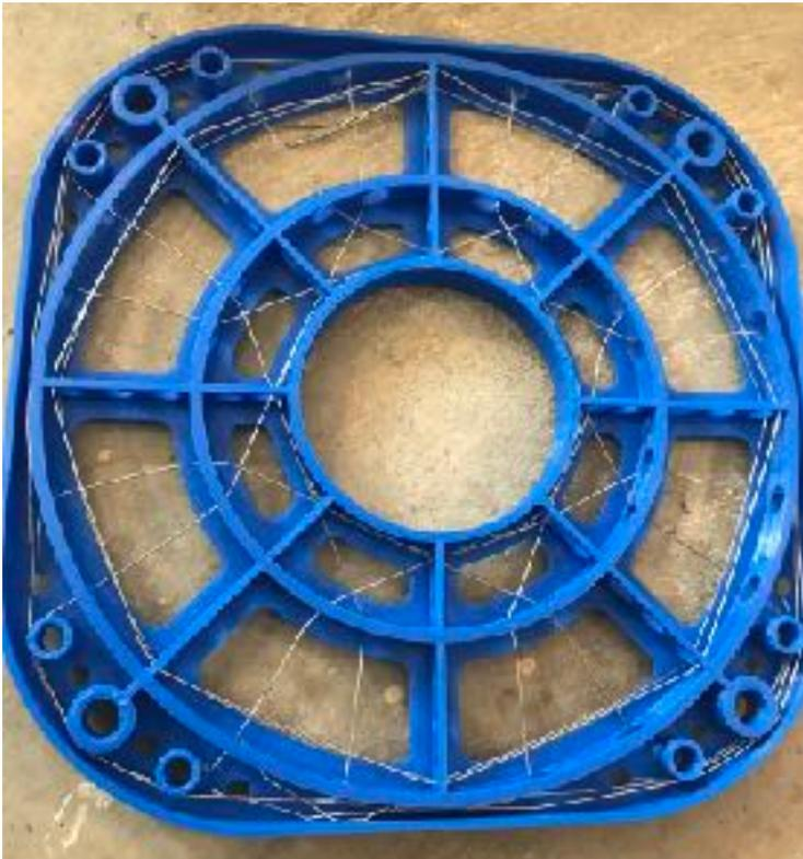
Next, I've used I've got a number of pieces of 22g galvanized steel wire as a reinforcing "fibre", and you can see how I've designed the ribs to have holes allowing me to string wire around inside the plate. I'm pre tensioning the wire a little, in the hopes of increasing stiffness.
