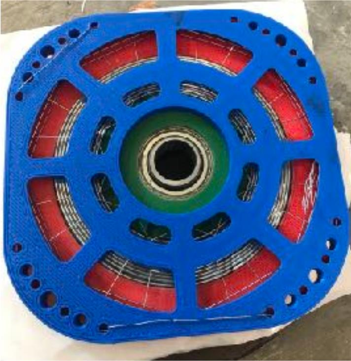
You can see in the blue plate, around the 3 through holes at each corner, I've got air vent holes, so that the poured in fill that coming next can fill around the bolts.
