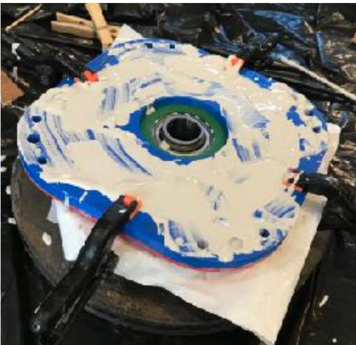
Here, I'm trying a new experiment. Super hard plaster of Paris (heavy repair 90, non sand-able, by Easy Fil, with about 50% PVA glue replacing half the water. Mixed fairly thick by hand, no chopped fibre, though that would also add a lot of strength, I didn't have any handy, and was worried it might keep the mix from flowing around bolt holes and into cavity around bearing shell.
